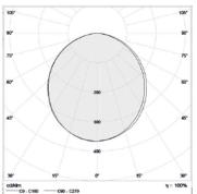
Correlated color temperature: 3000 – 6000 kelvin Rated median useful life: 50000h L70 at 25°C Luminaire input power: 12w
